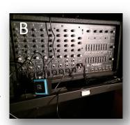
After switching on the system press the Bluetooth logo on the adaptor that is located inside the control panel this should already be connected into the "Line In" red and white audio sockets (see picture 'C').
